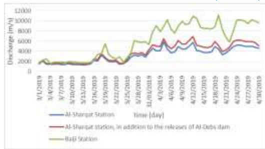
Fig. 21: Comparison of the hydrographs observed in Al-Shirqat, Baiji and Al-Shirqat (in addition to the releases of Al-Debs Dam) stations for the 2019 flood.
