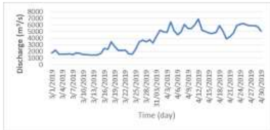
Fig. 13: The flood hydrograph observed at Al-Shirqat station, in addition to the discharge of Al-Debs dam, in March and April 2019.
