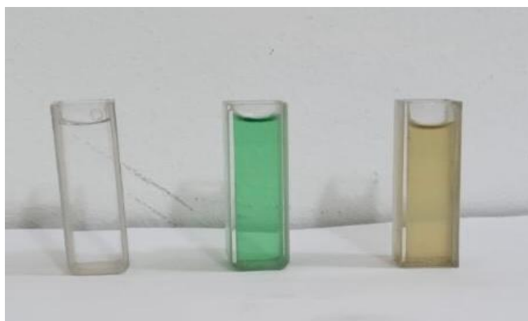
Fig. 2: Illustrative image of the samples used in the spectroscopic analysis, from left to right: the blank (non-ionic water), the NiO nanoparticle solution after the reaction, and the raw peppermint leaf extract before the reaction
